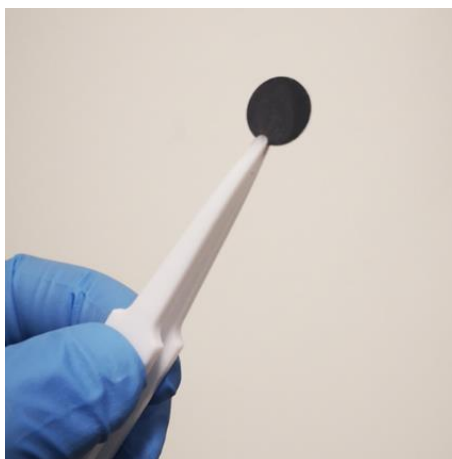
Figure S13. The MoS 2 pellets were compressed by 60 mg powder of each sample and were used to test electrical conductivity with the four-point probe equipment.
